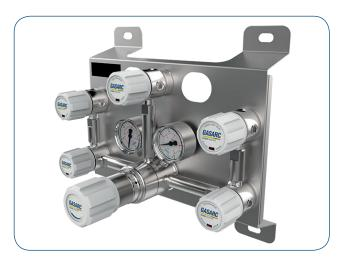
The Chem Master SGM6240 Series two stage twin cylinder manual change control panels are designed for primary pressure gas control of corrosive, toxic or high purity gases up to grade 6.0 purity (99.9999%), on gas distribution systems where constant delivery pressure is required.
