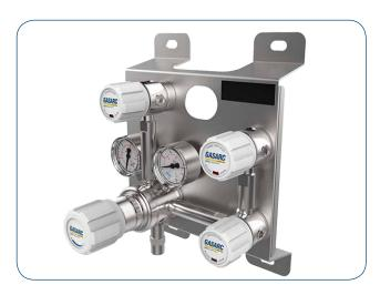
The Spec Master HPM6020 Series two stage single cylinder manual change control panels are designed for primary pressure gas control of non-corrosive or toxic, high purity gases up to grade 6.0 purity (99.9999%), on gas distribution systems where constant delivery pressure is required.
