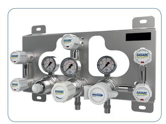
The Chem Master SGD6040 Series two stage differential autochange control panels are designed for primary pressure gas control of corrosive, toxic or high purity gases up to grade 6.0 purity (99.9999%), on gas distribution systems where constant delivery pressure is required.
